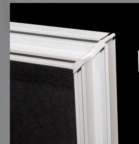
Our Patented Sash Glazed Double Hung Picture Window provides the exact same sight lines maintained within the same glass planes as our operable Double Hung units. This provides an aesthetic improvement over current window designs. Our Historic 1854 Ovolo Sticking (on 3/4" glazed sash), Putty Bead contours as well as the radius edge on the Sill Dam maintain the historic accuracy. With Performance Grade 50 ratings the Sanford Hills is as rugged as it is beautiful
